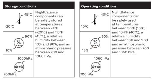
① The device is ready for use when within the operating conditions.
